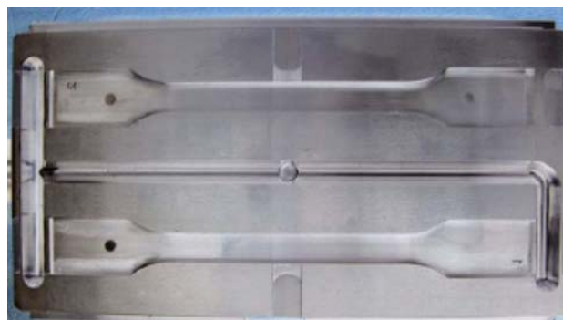
Fig. 1 Single- and double-gated cavities with nominal dimensions of 4 \times 10 \times 120 \text{ mm}^3 (thickness, width and length, respectively)
